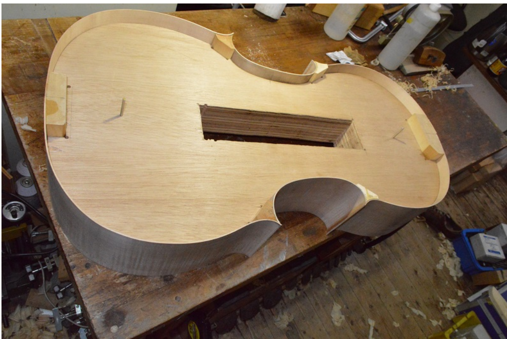
Picture 58 and 59: Bouts are complete.
