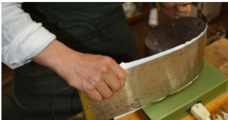
Picture 36 and 37: Bending a C-bout stripe.
