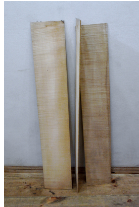
Picture 18: The boards that become the ribs of the final five-stringed cello. They are about 120cm tall. The board in the middle was turned by 90° in order to demonstrate how thin it is..
