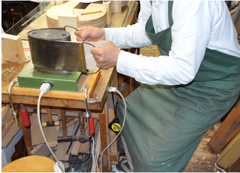
Picture 44: Bending of the shoulder bout.
