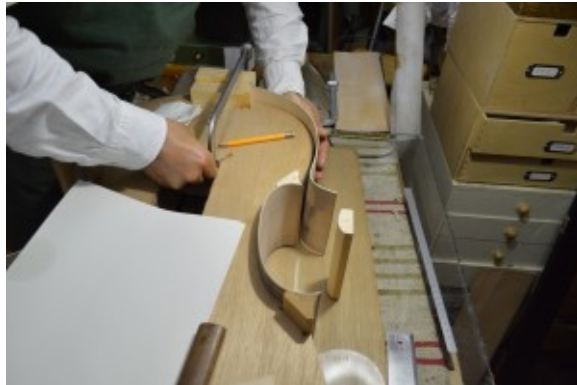
Picture 45 and 46: First fittings of the shoulder bout.
