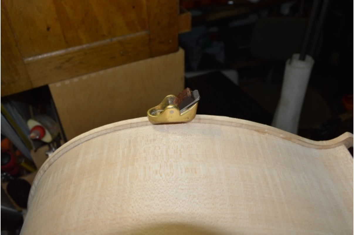
Picture 78, 79 and 80: The rim and the tools that are used for cutting it down. (Planing, filing, measuring.)
