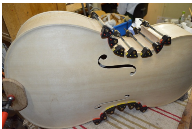
Picture 89: Top glued on.
