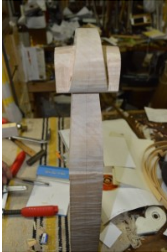
Picture 92 and 93: First states of producing the neck.
