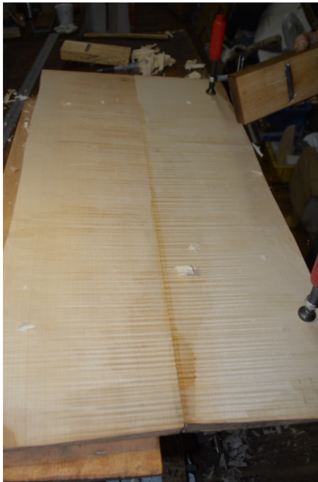
Picture 66: Back pieces glued together.
