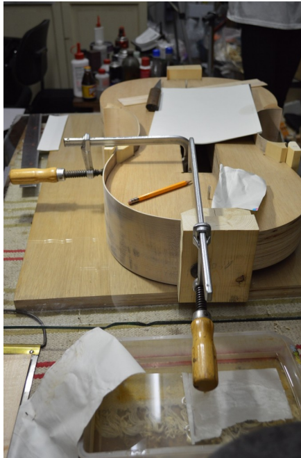
Picture 47: Positioning of the shoulder bout.
