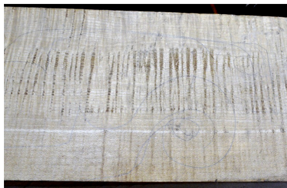
Picture 19: The block that will be used for scroll and neck. Ueda already roughly sketched the shape of the scroll onto it.
