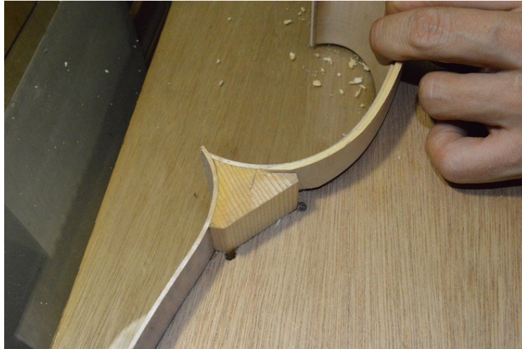
Picture 63: Opening a C-bout block before inserting the lining.
