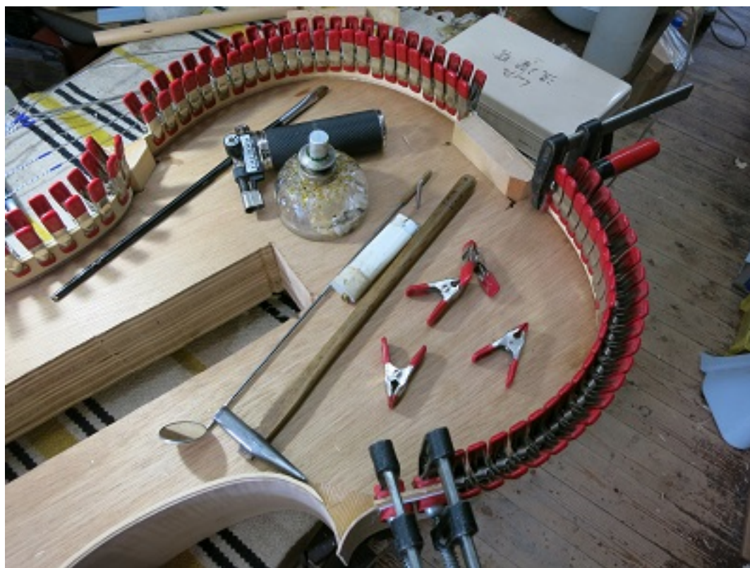
Picture 65: Shoulder lining in position.
