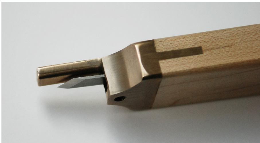
Picture 90: A purfling groove cutter.
