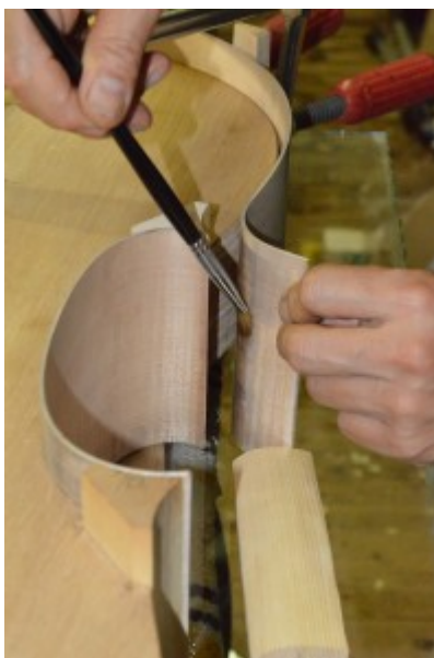
Picture 56: Putting glue on at the C-bout.
