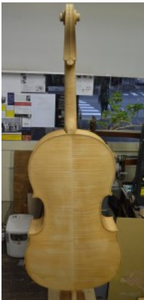
Picture 97: Body stained with coffee solution.
