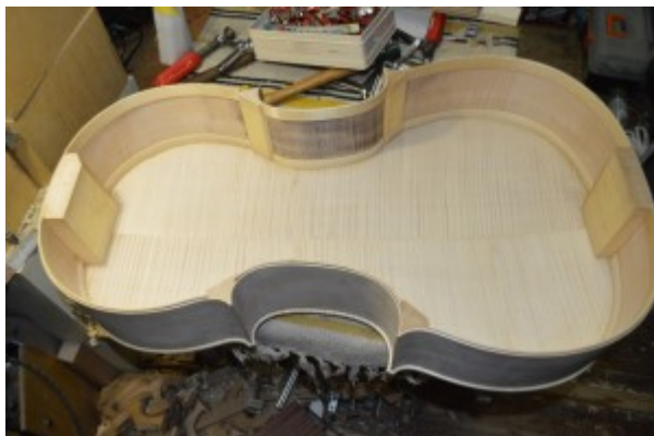
Picture 87: Form is removed.
