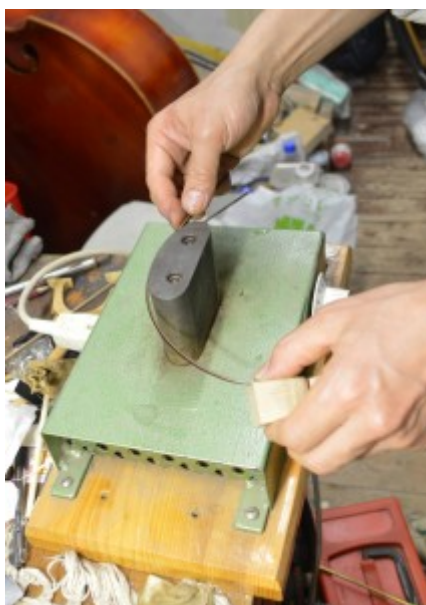
Picture 91: Bending of a purfling stripe.
