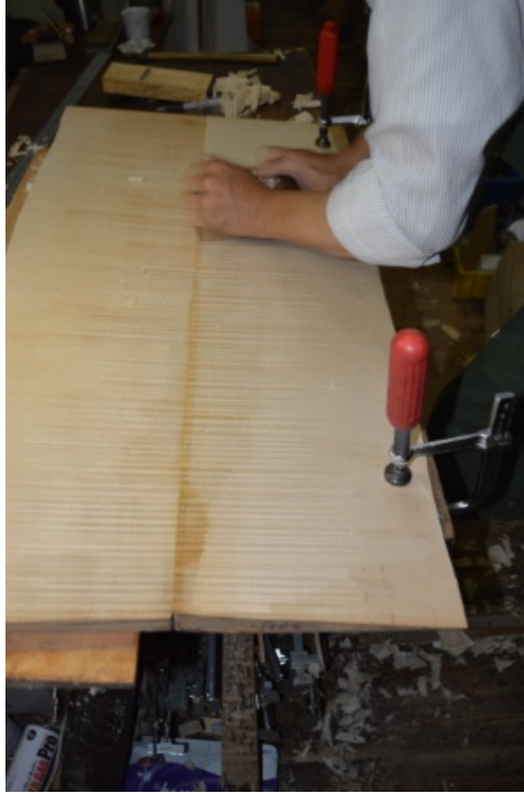
Picture 67 and 68: Planing and checking evenness.
