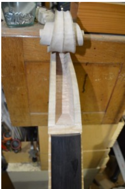
Picture 94: Fingerboard attached.
