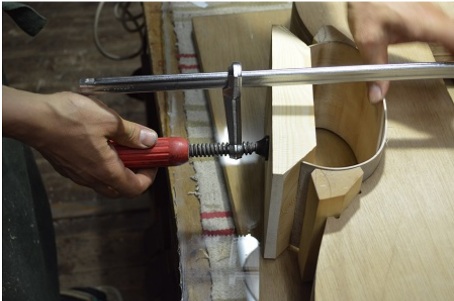
Picture 41: Fitting the C-bout into place.
