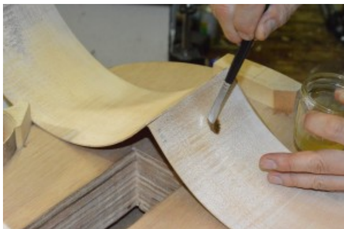
Picture 54: Applying glue to the neck bouts.
