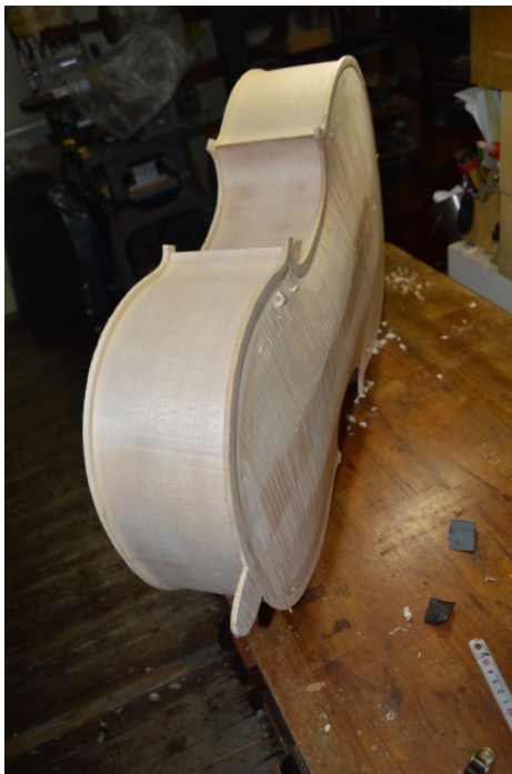
Picture 76 and 77: The temporarily glued-together body.
