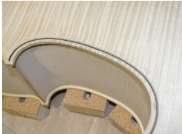
Picture 92: C-bout purfling put into place.
