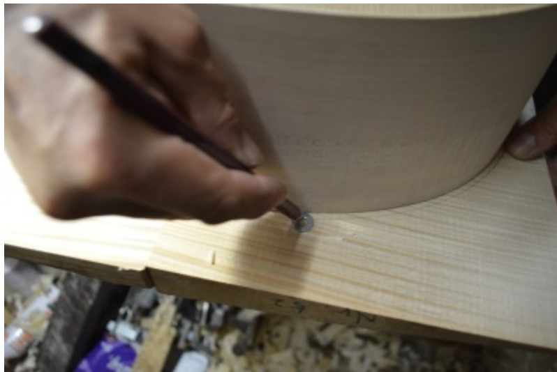
Picture 71: Drawing the contour of the edge.
