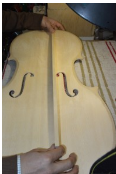
Picture 89: Fitting the bass bar onto the finished top.
