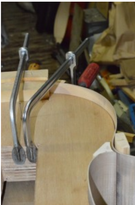
Picture 55: Fixing bouts to the neck end.
