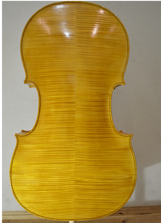
Picture 100: Back after third layer of front varnish.
