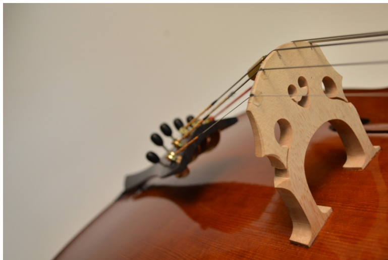
Picture 102: The finished bridge.
