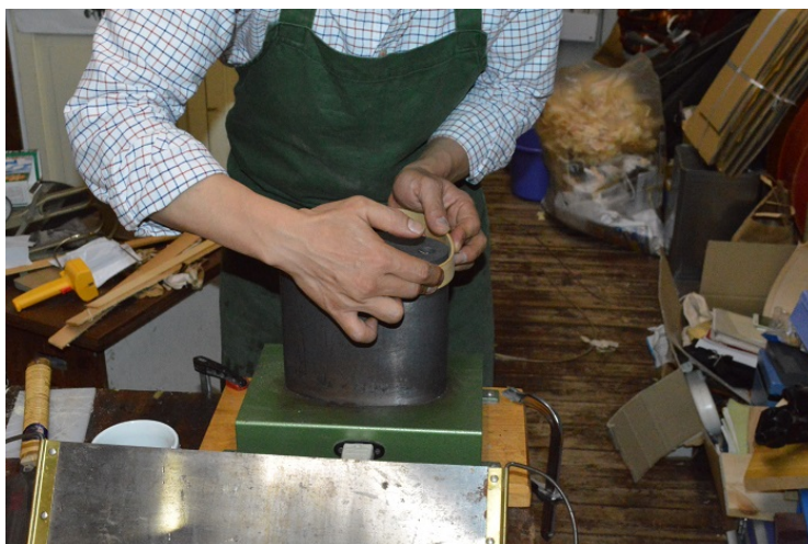
Picture 62: Bending a C-bout lining.
