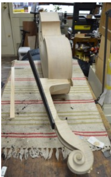
Picture 95: Provisionally attached neck.
