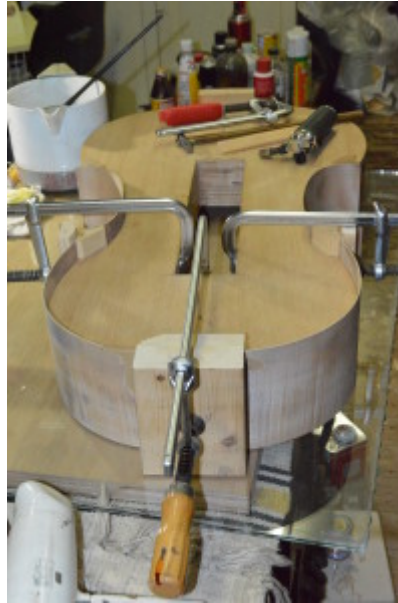
Picture 57: Both upper bouts are fixed into place.
