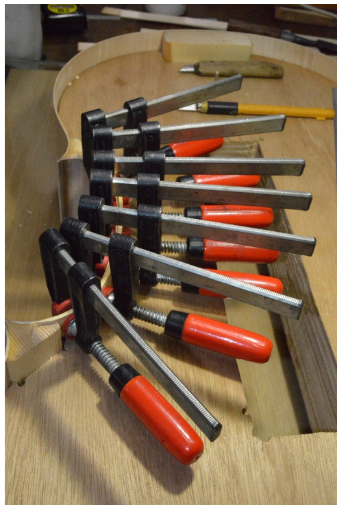
Picture 64: Fitting-in of the lining of a C-bout.
