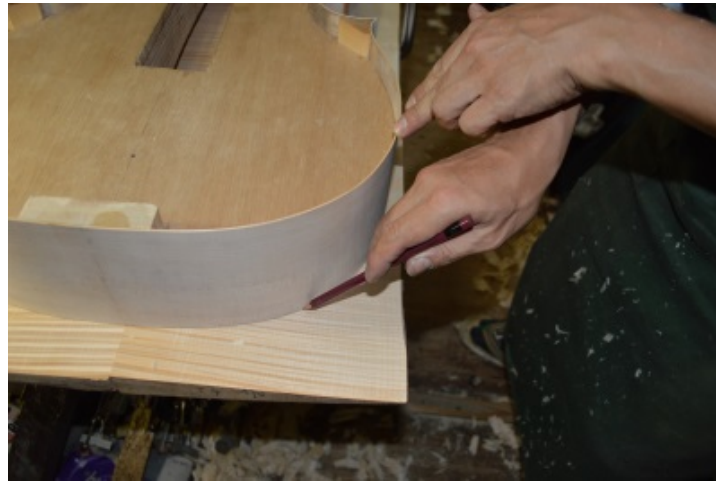
Picture 70: Transferring the contour of the bouts.
