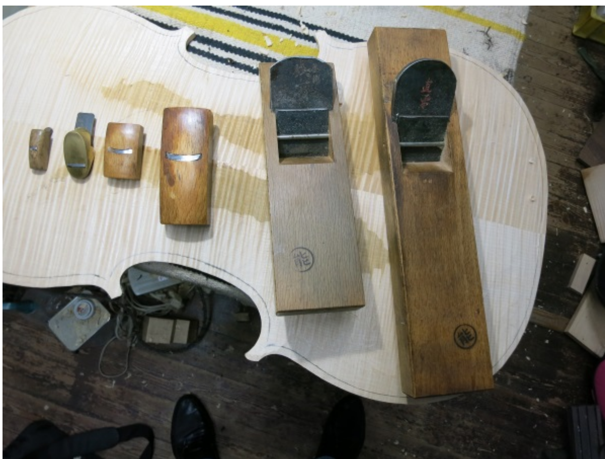
Picture 76: Some of the tools used in the planing-, arching process.
